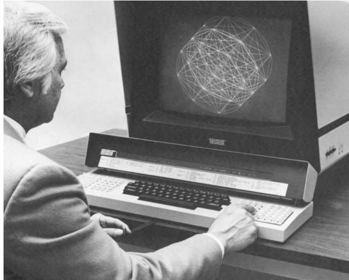
Figure 21.6 Gerber IDS-80 Storage Tube Terminal (Note lever under keyboard used to control cursor and the two 40-button function keyboards bracketing the alphanumeric keyboard)
