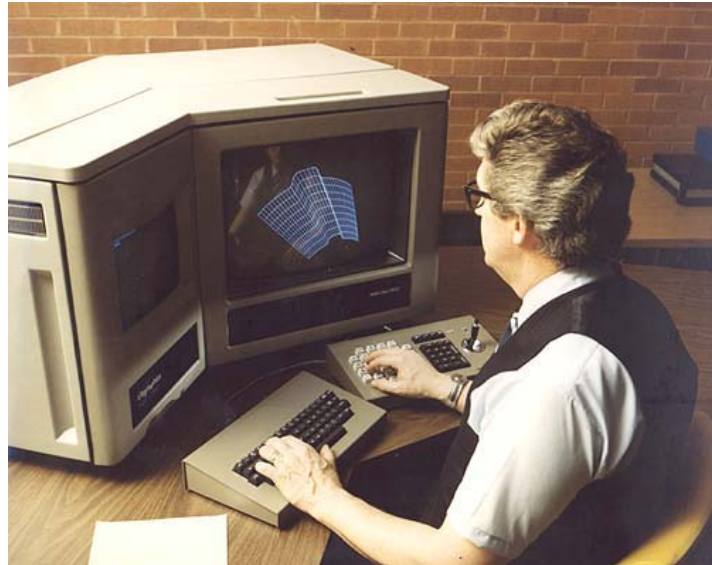
Figure 19.6 D-100 terminal showing keyboard and program function keyboard (PFK) 7
