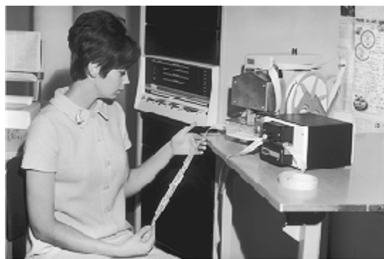
Figure 19.3 DEC PDP-8 based UNIAPT System
